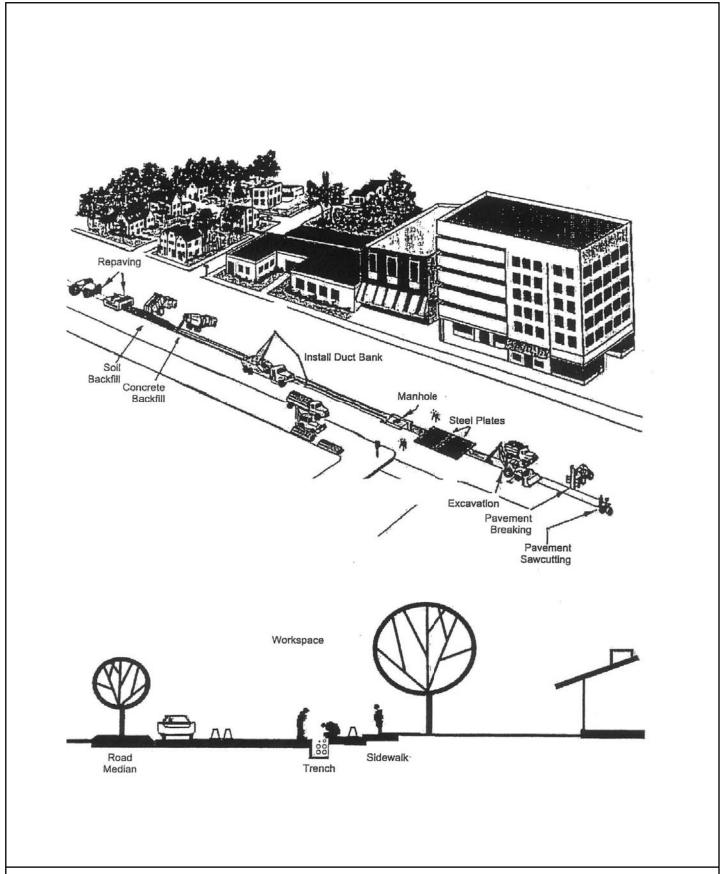
Source: SDG&E,2014 Figure B.1-20: Typical Underground Construction Process within Roadways
